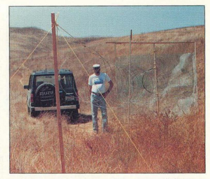
Photo A. Gary Holoubek WB6GCT (pictured) and Tony Levand KA9WGO assembled this 16' long circularly polarized beam with a 6' x 6' screen reflector in a wilderness park for a Fullerton Radio Club T-hunt. It put lots of RF at the far end of the canyon, but very little signal at the road just behind it.
